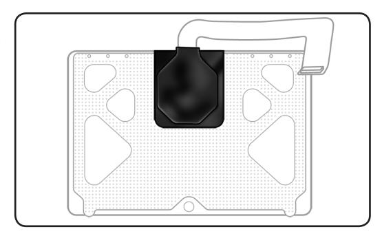
2 Align new flexures on positioning posts.
