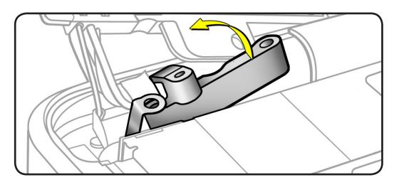
Replacement Note: Be sure grounding clip fingers contact the small top case pocket.
