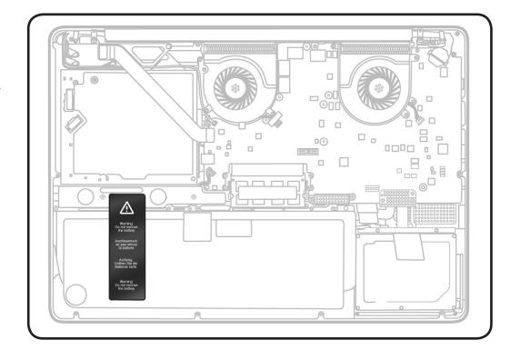
**5** Without pulling cable, tilt out battery.
