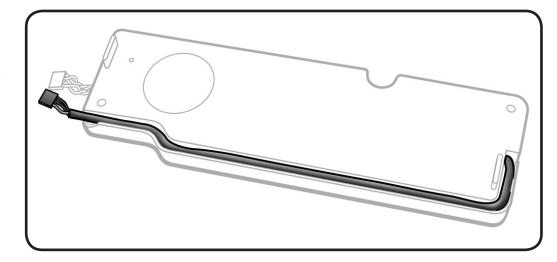
**2** Turn over speaker, and carefully pry up the microphone gasket.
