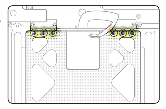
**8** On the palm rest, insert one sticky (Post-It) note into gap on each of the four sides of trackpad.
