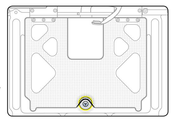
**14** Adhere flex cable to mounting ramp.
