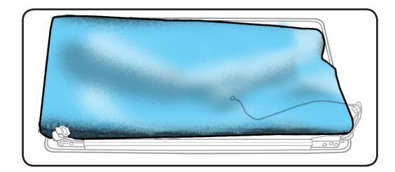
**2** Holding left hinge, slide clutch cover 1/4 inch (6.35 mm) away from the LVDS cable.
