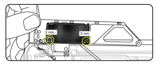
Replacement Note: Make sure connectors are fully seated, and the length of the cables are tucked into their channels.
