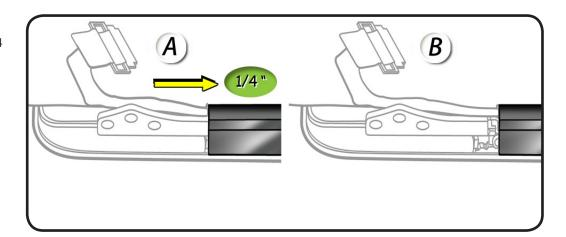
**3** Press down on clutch cover to loosen 4 hooks inside.
