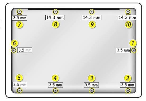
Use black stick to loosen and remove bottom case.
