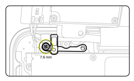
Remove the camera cable guide.
