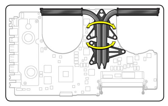
**3** With a black stick, scrape off thermal grease and use alcohol pad to clean thermal pads and chips.
